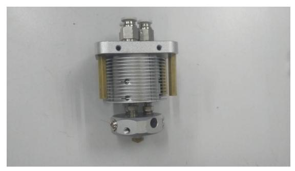
There is a print head fixing platform on the printer. Let the lower part of the print head through the circular hole of the platform and use 4 M3\*16 cylindrical head bolts to fix the bottom (details see pictures below).
