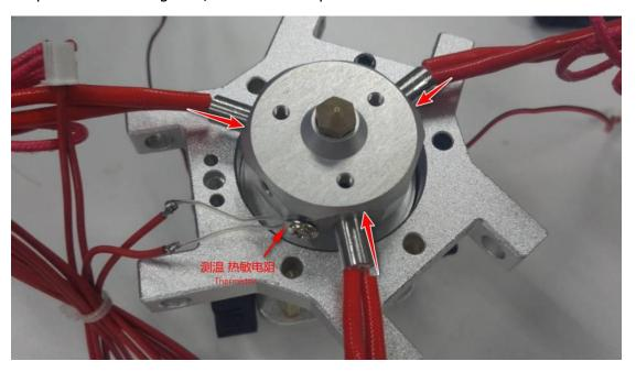
Connect the wires of heating rod, fan and thermistor, and put the teflon tube into the quick connect plug. You can use it now.
